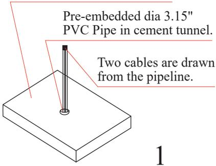
Drill 4 holes in the cement pier(4-dia0.55") Drill a hole that is 4.73" deep.
